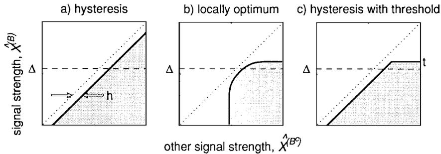
Fig. 2. Decision regions based on the predicted signal strength  $\hat{X}^{(B)}$  of the current station and the other station  $\hat{X}^{(B^c)}$ , respectively, for three different handoff strategies. Decision in favor of handoff is made when the signal strengths lie inside the shaded area.
