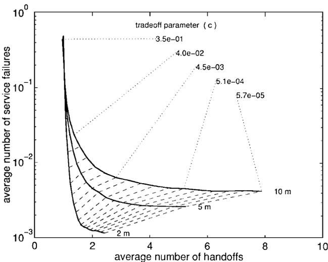
Fig. 4. Tradeoff curve parametrization. Performance of the locally optimum test is shown at sampling distances corresponding to mobile speeds 14.4, 36, and 72 km/h (assuming  $t_s = 0.5$  s). Dashed lines connect points of the equal tradeoff parameter. Unlabeled tradeoff values are spaced logarithmically between indicated values.
