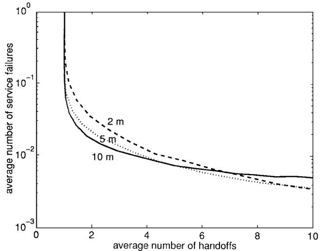
Fig. 5. The hysteresis algorithm does not adapt to speed. Performance of the hysteresis test is shown at sampling distances corresponding to mobile speeds 14.4, 36, and 72 km/h (assuming  $t_s = 0.5$  s). Compared with the locally optimal test (Fig. 4), the achievable performance of hysteresis tests is relatively unchanged at different mobile speeds.
