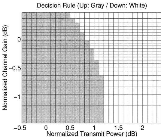
Fig. 2. Graphical display of the optimal binary single-user power control policy. As the link quality improves, the mobile unit reduces its power consumption.
