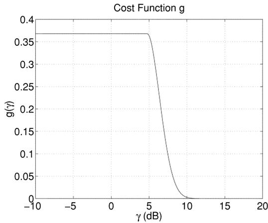
Fig. 1. Plot of the cost metric  $g$  as a function of SIR. A low SIR induces a high penalty, while a sufficiently high SIR yields no cost.
