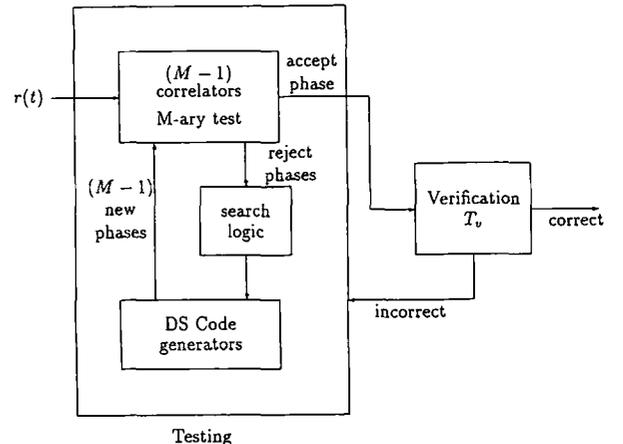
Fig. 1. Structure of hybrid acquisition schemes.
