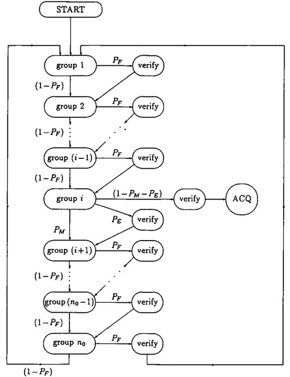
Fig. 2. Block diagram of hybrid acquisition schemes.
